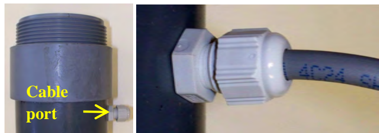
Figure 11. Cable port located near top of enclosure (left) and detail (right).
